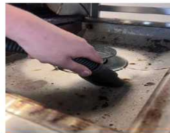
Vacuum around the ceramic base, burners and ignitors
